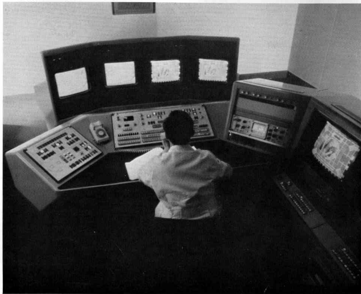
Below: Main control suite in the new London colour control and monitoring centre at Croydon
