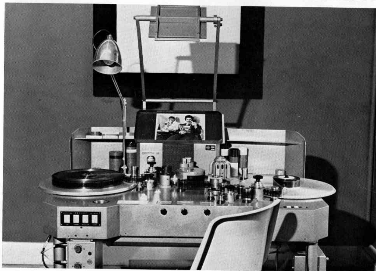
Below: Prevost film preview table: Dual 35/16 mm. Accepts Spools or Rolls up to 3,000 ft 3-speed operation, forward and reverse. Large or small screen capability
