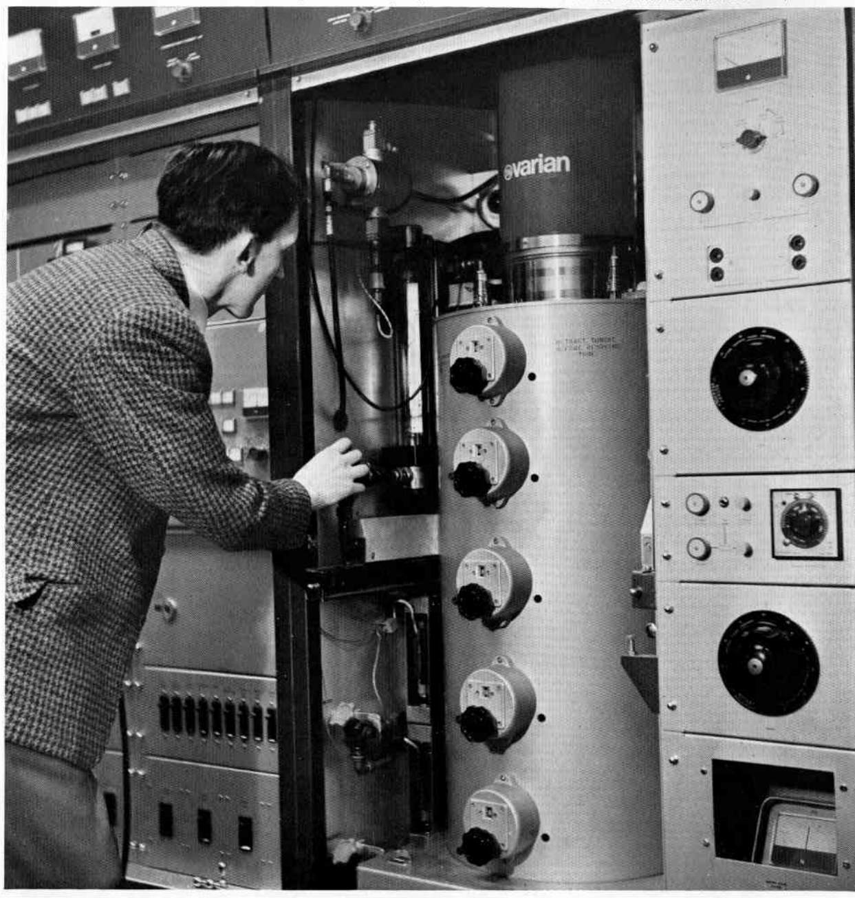
An integral five-cavity Klystron installed in one of the 40 kW transmitters at Crystal Palace
